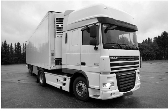
Figure 1.2: DAF XF prototype heavy-duty hybrid electric truck with a parallel topology.
