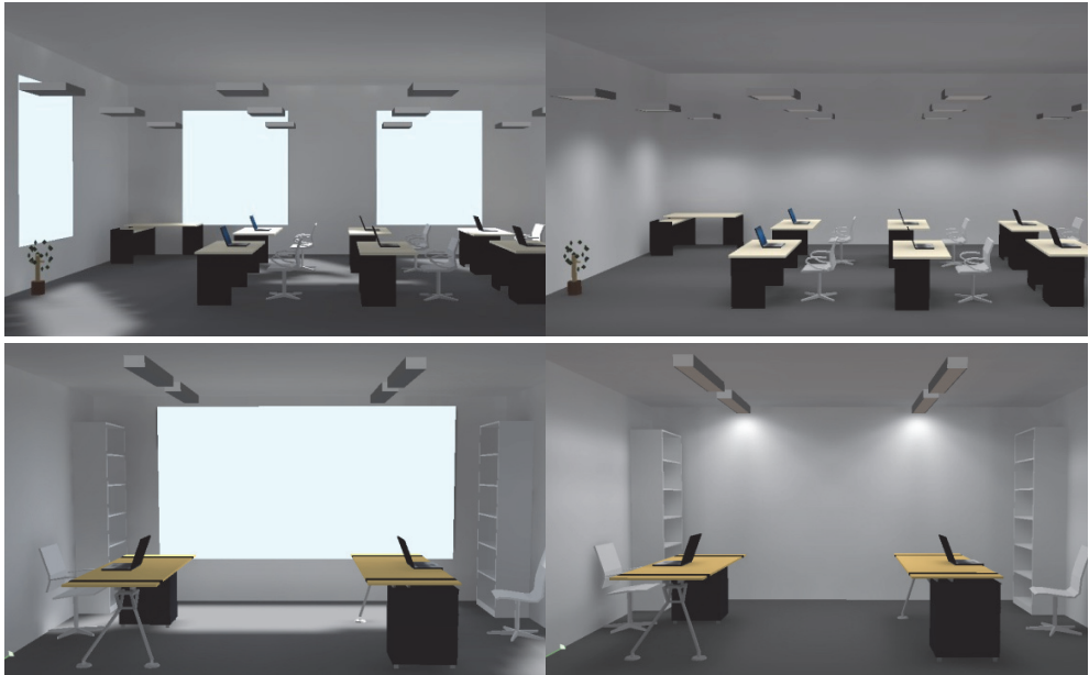
Figure 4.1 Virtual environments used in the daylight (left) and electric light (right) conditions.
