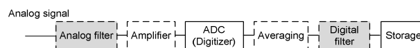
Fig. 1. A typical AD conversion process; the dashed blocks indicating additional filtering and amplification as well as signal averaging are optional; either analog filter or digital filter can be applied in one system
