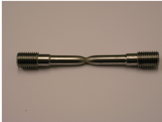
Figure 1: A neck appears after applying a critical load to the cylinder.
