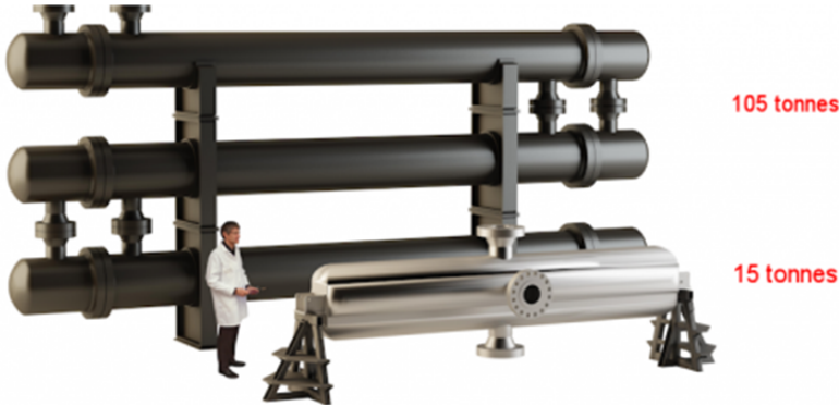
Figure 8.6. Size and weight comparison of a PCHE (front) and a shell and tube heat exchanger for same duty 28
