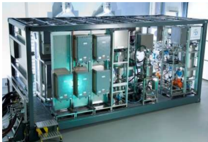
Figure 1.6. Bayer's Process Equipment Container Unit installed at INVITE (from F 3 Factory newsletter 174 )
