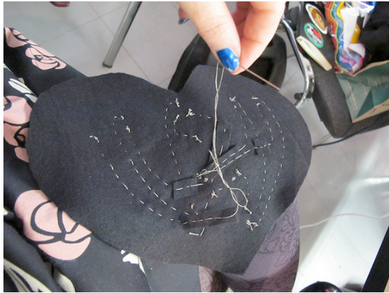
Figure 3. Sewing of conductive thread seen from the underside of the design
