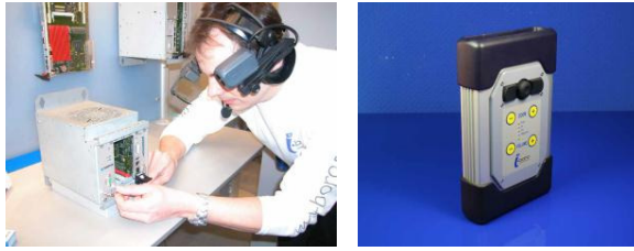
Image 1: i-boro wearable PC for remote service technicians
