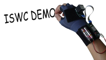
Figure 1. System usage illustration showing the wireless data glove with all components.
