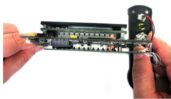
Image 3 – teXXmo ONE three-layer architecture
