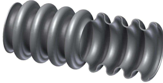
Figure 1.1: A short segment of a typical corrugated pipe, showing a longitudinal cross section of the corrugated wall
