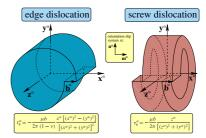
After employing these back-stress relations to determine the resulting stress in the origin of a dislocation field (represented by the dots in the figure below), only GND density *gradients* appear to play a role:
