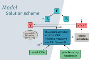
To implement this scheme into a FE environment, each grain is subdivided in finite elements, where up to 18 GND densities are considered as additional nodal variables.
