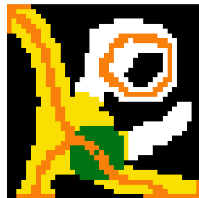
FIG. 5. (Color online) The backbone (BB), shown in yellow, is the union of maximal disks centered on the percolating part of the Skeleton by Influence Zones with boundary (SKIZb), here shown in orange. For the green SKIZb-pixel the maximal disk associated with it is shown.
