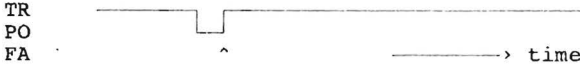
Figure 5.3. The rule's conclusion may have been true at all times, but at some time it was impossible to establish its conclusion. The history counter reflects the time, indicated by the arrow, where the conclusion last changed. The history operator erroneously returns FA rather than PO.
