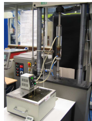
Figure 1 a) The applied stress signal. b) The isothermal set-up.
