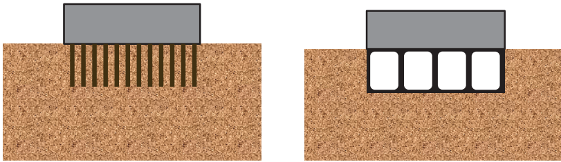
Figure 7: Two different types of foundation: (concrete) pillars or a very light structure.
