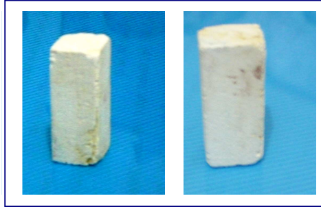
Figure 4. Cement samples from cement systems produced at 1350 °C with different water ratio. (a) 0,50 ratio; (b) 0,85 ratio.
