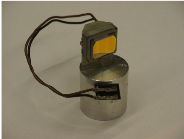
Figure 5.6. VLP scanning mirror used in the high-resolution deflectometer. The scanning aperture is 10 x 15 mm and the resonant frequency 50 Hz.
