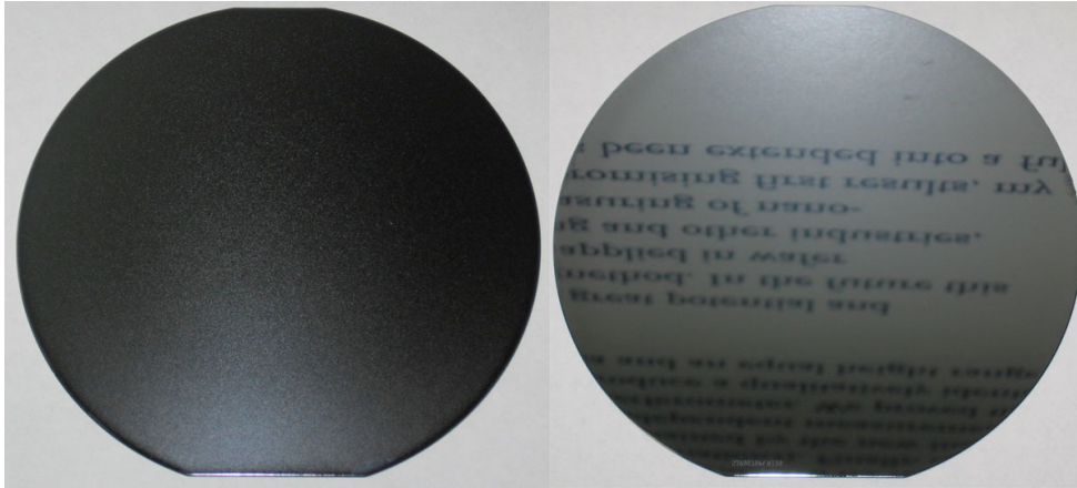
Figure 4.4. A silicon wafer with a rough, grinded surface (left) and with a specular, CMP-polished surface (right).
