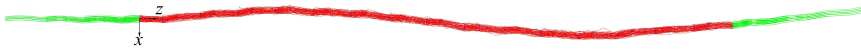
Figure 6.16: Simulation snapshot. Side view of the relaxed unloaded crystalline fibril obtained after the simulation. The wavy profile displayed is in fact right-handed writhing of the bundle as also evidenced by the end view of this same fibril state displayed in Figure 6.17. Note that the profile of the fibril before the start of the simulation was perfectly straight. The portions of the fibril near its ends (those colored green) where not allowed to thermally relax. Each portion is of length 4.5 \times 67 nm along the fibril. The left end is the grafted end.
