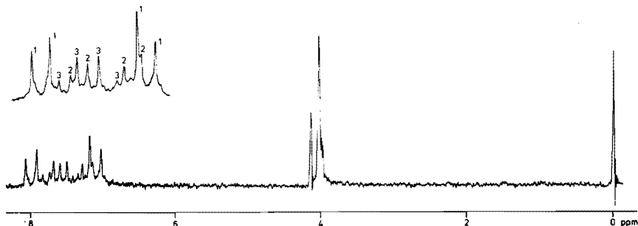
Fig. 3.5 4-deutero-1,2,3,4-tetra( p -methoxyphenyl)cyclobutyl cation in \text{CF}_3\text{COOD} . Shifts in ppm downfield from TMS.
