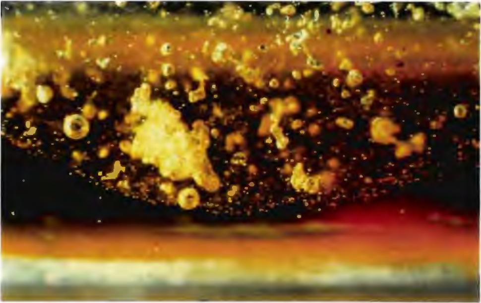
Figure 6.22: Air bubbles in a porous medium, submerged in a 1.35 g/ml NaI saline solution. The picture covers a width of the porous medium of about 16 mm.
