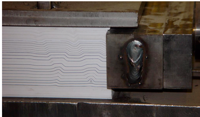
Figure 7: An experiment similar to that of Fig. 5, in which the foam is replaced by further sheets of paper, creating a much stiffer confinement. As a result the kink bands are shorter and more orthogonal to the layering. Experiment performed by Ahmer Wadee at Imperial College, London [10].
