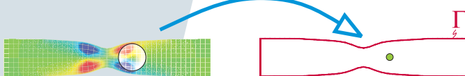
Figure 2 Schematic representation of the non-local interactions. The internal length \ell controls the degree of non-locality.
