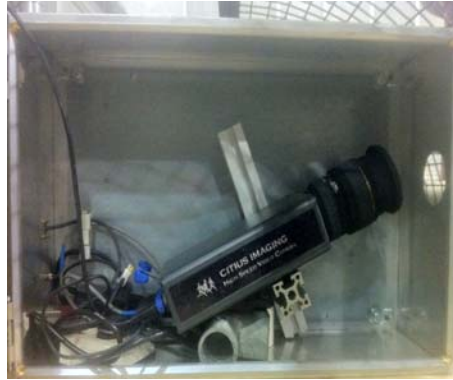
Figure 4.14. High-speed camera for recording the arc image in a shielding box.
