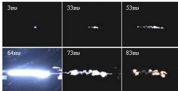
Figure 7.5. Arc images at characteristic instances from a successful current interruption. The time of the Figure 7.5 corresponds to the time of Figure 7.4a.
