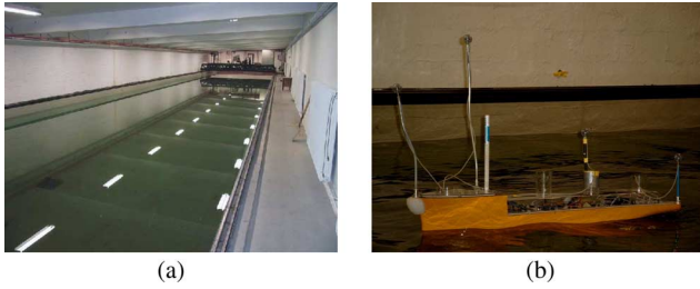
Fig. 1. Marine Cybernetics Laboratory, Tyholt, Trondheim. (a) Basin. (b) Cybership II, a model supply ship, Froude scaled 1:70.
