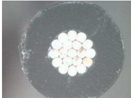
Figure 5.7: 19-core SI-POF, product model: SMCK-1000 from Asahi Kasei (illuminated by white light).
