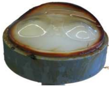
Fig. 7 After the measurement series, the outside radius of the sample has been affected by corrosion of stainless steel. Dissolved iron ions ( \text{Fe}^{2+} or \text{Fe}^{3+} ) bind to the ionized groups (fixed charges) of the polymer gel, leading effectively to a decreased fixed charge density in the outer shell of the sample.
