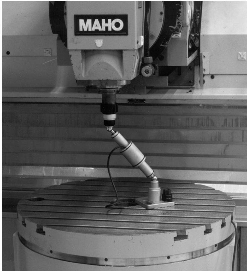
Figure 1.3: A telescopic Double Ball Bar (DBB) measurement on a five-axis milling machine.
