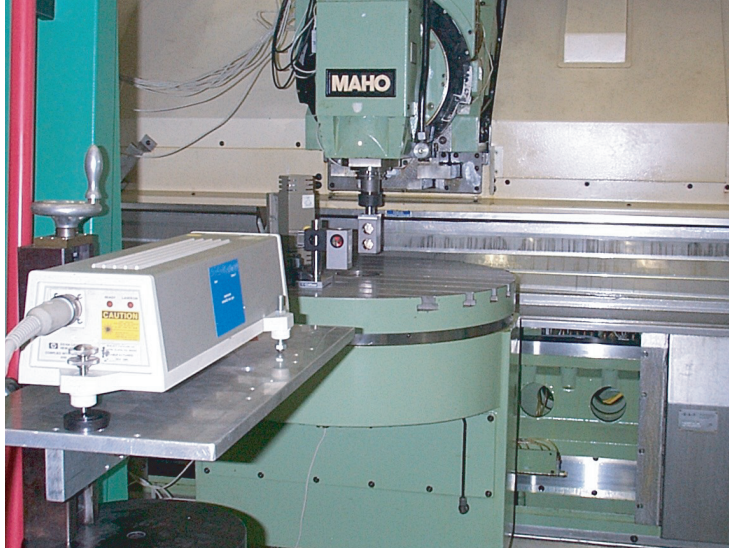
Figure 4.7: Direct measurement of error component zrx using a laser interferometer.
