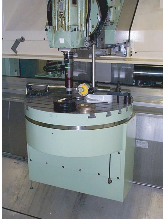
Figure 3.10: Measurement setup for determining the lateral stiffness of an extended tool.
