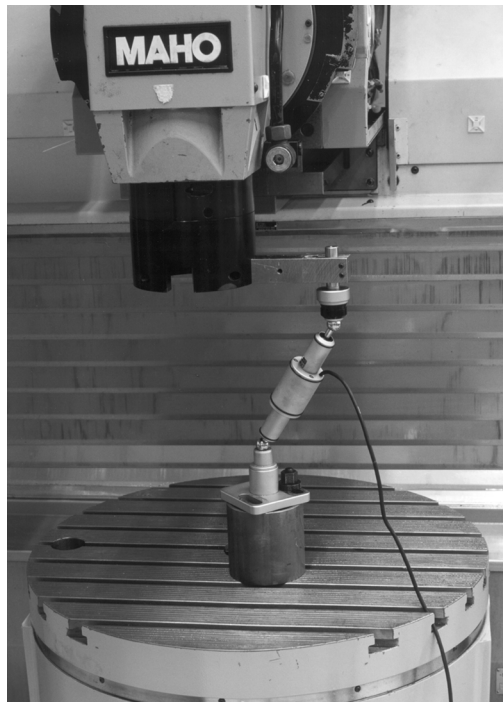
Figure 3.9: DBB measurement with offset adapter and elevated stand.
