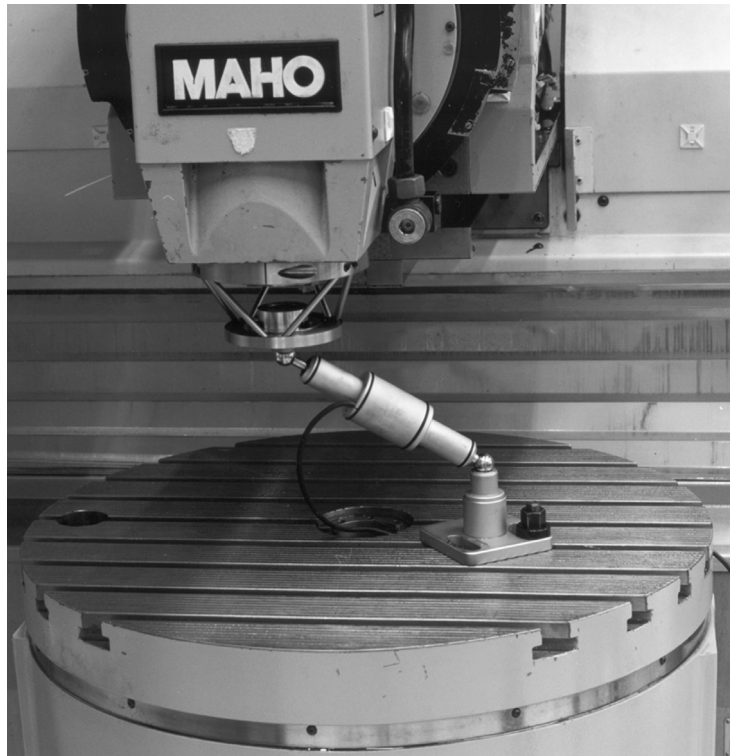
Figure 5.9: Photograph of a DBB measurement setup for determining thermally induced errors, using the developed adapter.
