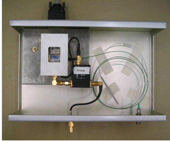
Figure 3.3: RSOA with MQW material [62].
