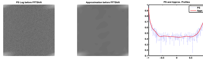
FIGURE B.1: A tin balls sample: power spectrum, its approximation and their profiles before the shift.
