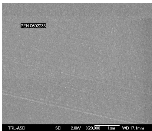
Figure 4. SEM image of the APGD deposited silica-like film on PEN substrate
