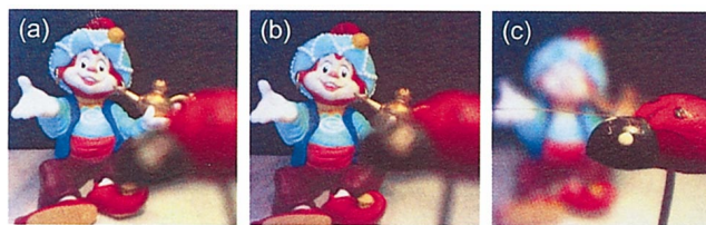
FIG. 4. (Color) Frames taken from a video made with a VGA CMOS camera having (a) a fixed-focus lens and (b) a liquid lens focused at 50 cm and (c) a liquid lens focused at 2 cm.
