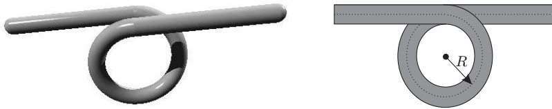
Figure 3.7: Configuration of a two metre fibre with one single loop of R = 14 \text{ cm} to obtain \lambda_{ce} .
