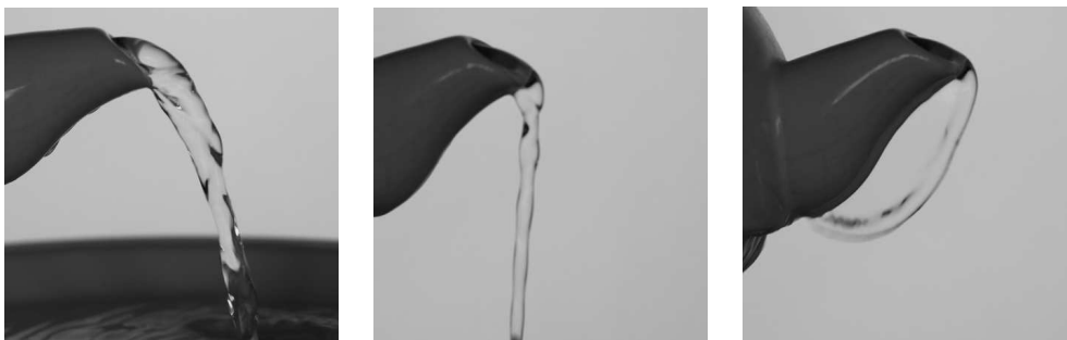
Figure 1.12: The teapot effect: if one fast pours water from a teapot the water stream resembles a ballistic trajectory (left photo); if water pours a bit slower the water stream is vertical (middle photo); if water pours very slowly, the water clings to the underside of the teapot lip (right photo);
