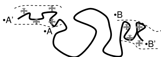
Figure 4.6: Schematic picture of the heterogeneous melt. The melt consist of entangled (AA' and BB') and disentangled domains (AB). The de Gennes' virtual tube required for the cooperative reptation is absent in the disentangled domain since it is depleted with entanglements.
