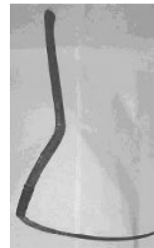
Figure 4. Finnish väärävirtinen viikate , bended scythe, provides information for the user how to adjust it with the users body and movements.
