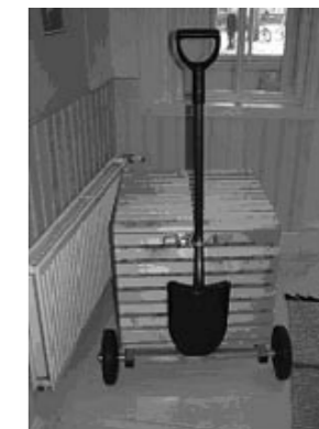
Figure 2. This garden carriage was designed so that the shovel would serve as the handle to push the carriage around. In a usability test users did not understand this function but took the shovel off and started to use it with normal swinging movement.
