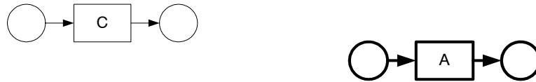
Figure B.18: STEP 1b: A transition with an input and output place is added for data element A.
