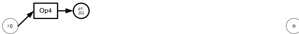
Figure B.47: STEP 3a: The first execution path \sigma_1 is selected and its operations are added to the model stepwise. The first operation that is executed in this execution path is Op4 . A transition Op4 and an output place p1 representing the situation in which a value for the output element of operation Op4 , i.e. C is available, are created. The input place i is connected to transition Op4 and transition Op4 is connected to place p1 .
