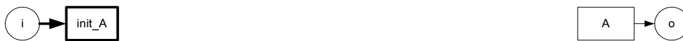
Figure B.3: STEP 2: Data element A is not a leaf element and can be produced by more than one operation. Therefore, a transition init_A is added. The ingoing arc to transition A is redirected to transition init_A .
