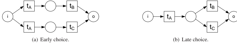
Figure 5.3: Both process models in (a) and (b) have the same set of firing sequences, i.e. S = \{\langle t_A, t_B \rangle, \langle t_A, t_C \rangle\} . However, in the first example (a) it has to be decided before t_A is executed whether t_B or t_C will follow on the execution of t_A . In the second example (b), this choice is deferred to the moment when t_A has been executed. We say that the moment of choice in the first model is early, and in the second model is late.
