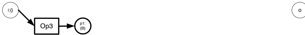
Figure B.36: STEP 2: One of the leaf operation is selected: Op3 . A transition Op3 is created for this operation, together with an output place p1 representing the the availability of a value for data element B . Place i is connected to transition Op3 and transition Op3 is connected to place p1 .
