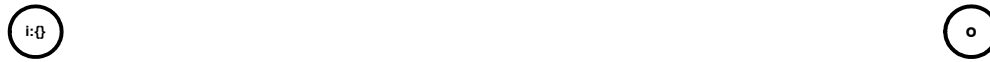
Figure B.35: STEP 1: An input place i and an output place o are created. The input place i represents the situation in which no data element values are available, denoted by \{\} .
