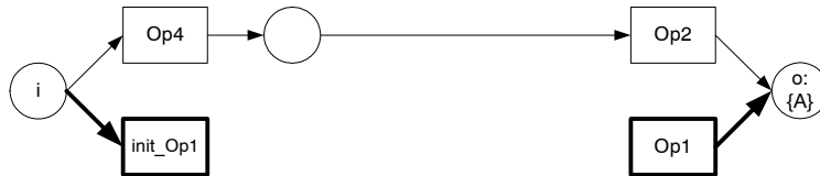
Figure B.12: STEP 4: Now operation Op1 is selected because it produces a value for A . Transition Op1 is added to the model and connected with place o . Since operation Op1 has more than one input element, also a transition init_Op1 is added. Place i is connected to init_Op1 .
