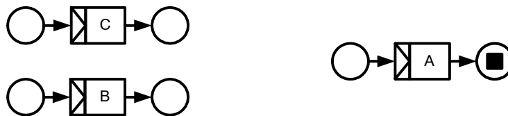
Figure B.23: STEP 1: A task with one input and one output condition is added for every data element in the PDM (cf. STEP 1 of algorithm Charlie in figures B.17-B.19).
