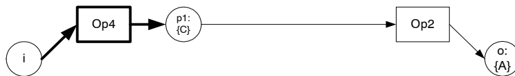
Figure B.11: STEP 3: Operation Op4 is selected because it produces data element C . Transition Op4 is added and connected to place p1 which represents the availability of a value for C . Since operation Op4 does not have input elements, the input place i is connected to transition Op4 .
