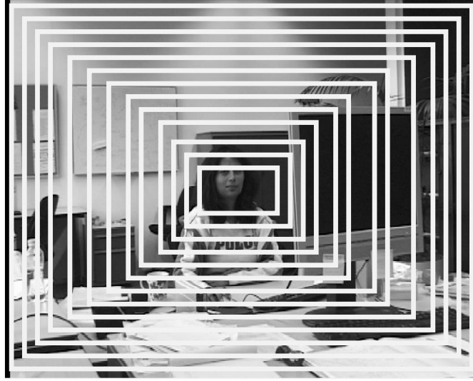
Figure 3.12. Concentric rectangles along which pixels are averaged.
