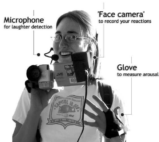
Figure 2.2. The camcorder “LafCam” implements three affective input channels [Lockerd and Mueller, 2002].
