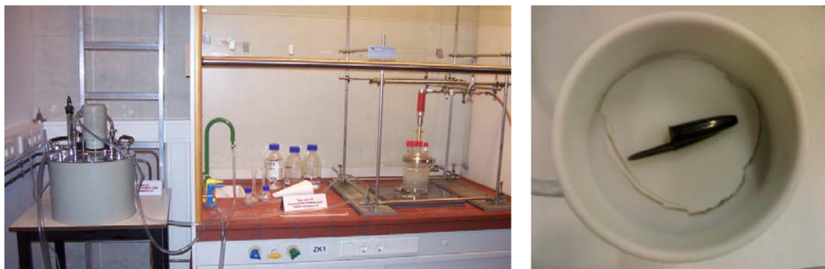
Figure 4. A) Lab scale setup for the production of olivine silica. Figure 4.B) Nano-silica produced in a stirred reactor at 70 °C and with a 3M sulphuric acid.
