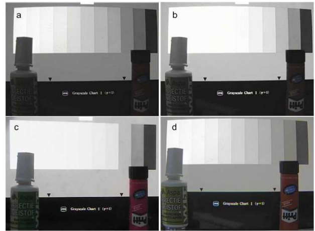
Figure 5: Results: (a) standard camera image, (b) smart extended range Gamma, (c) method from the Ref. [3], (d) our method ( a=0.5 ).
