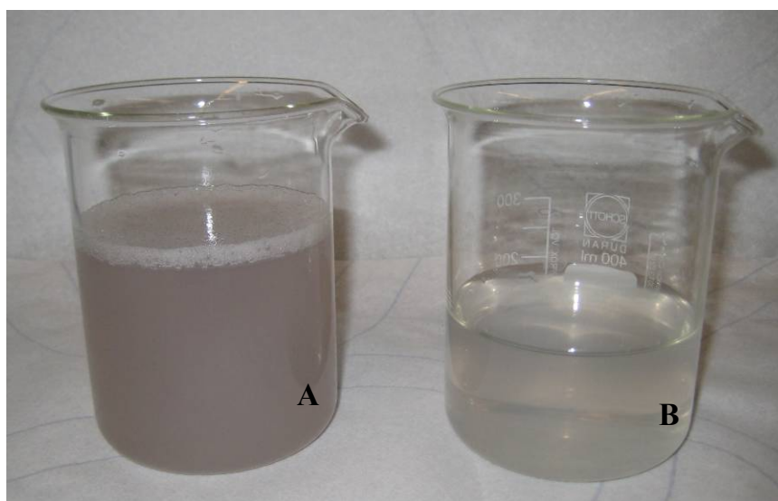
Figure 3: A. model rinsing water and B. treated water with the bucket-to-bucket prototype.
