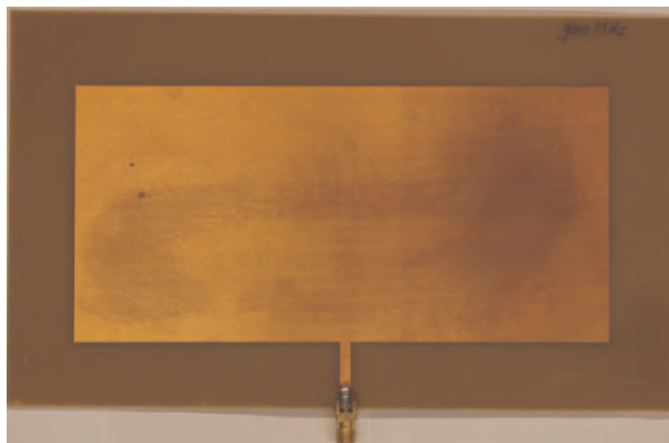
Figure 4.58 Microstrip patch antenna with microstrip line feed matched to 50\Omega
