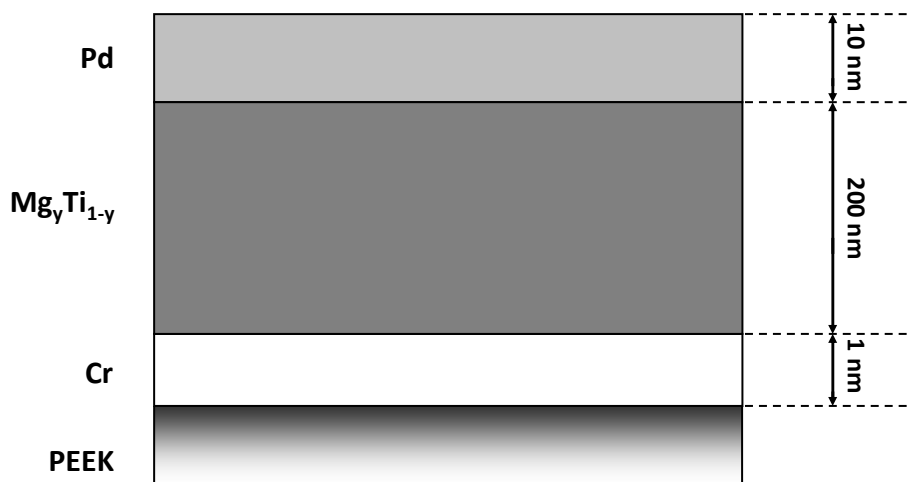
Fig. 2.16 Schematic representation of the layered structure of a 200 nm thick \text{Mg}_y\text{Ti}_{1-y} thin film alloy capped with a 10 nm thick Pd layer deposited on PEEK using a 1 nm Cr adhesion layer.
