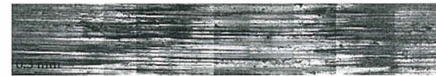
FIGURE 11.16 (See color insert.) Metal surface after the lubricity test for lubricant W.
