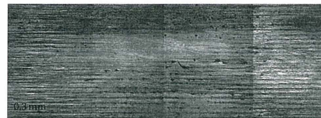
FIGURE 11.19 (See color insert.) Metal surface after the lubricity test for lubricant S2.
