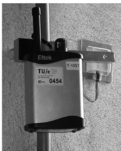
Figure 3. Measurement of the surface temperature and relative humidity using a box
