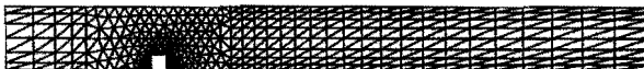
Fig. 3.16 : Finite element mesh as used in the unsteady flow calculations (660 elements, 1445 nodes).
