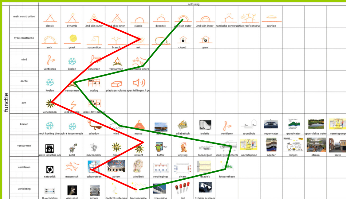
Morphological Overview for Adaptable Roofs; the red en green lines give possible combinations for possible solutions / concepts
