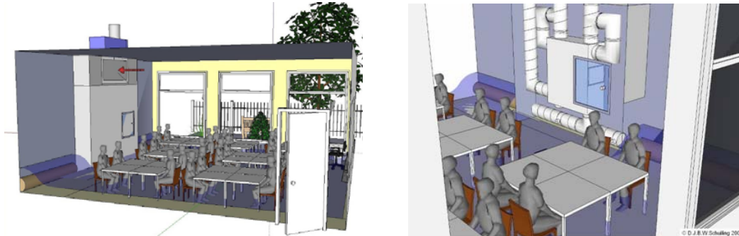
Figure 5. Example of the investigated displacement ventilation prototype as applied by Schuiling (2008).
