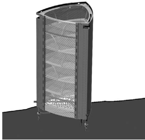
Figure 3: Food dehydrator designed for Haiti that responds to Haitian worldview, culture and context. Primary design influences: distribution by donkey and foot path, locally available materials, skill set of local labor, and economic development.
