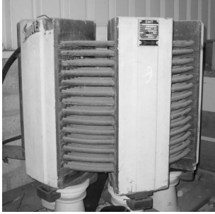
Figure 3.19 Photo of air core reactor manufactured by Smit and technical information on the two tested reactor models.
