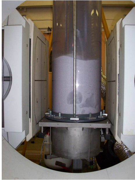
Figure 4.3: A typical PEPT measurement, bed filled with glass beads, superficial gas velocity of 1.5 u_0/u_{mf} and packed bed aspect ratio of 1.
