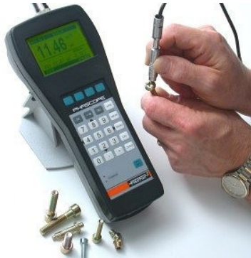
Figure 1.13: Zinc layer thickness using a leptoskop measuring device (=thick layer scale)
