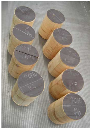
Figure 2.44: Core samples (diameter 80mm) from laminated timber beams
