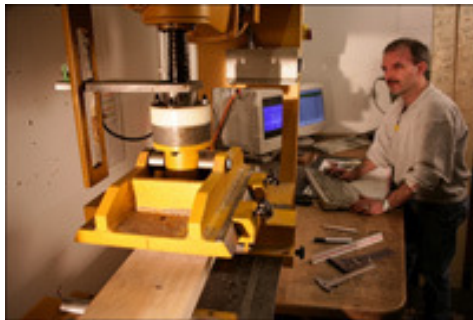
Figure 1.12: Finger joining inspection
