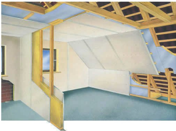
Figure 2.28: Gypsum plasterboard covering on a roof extension
