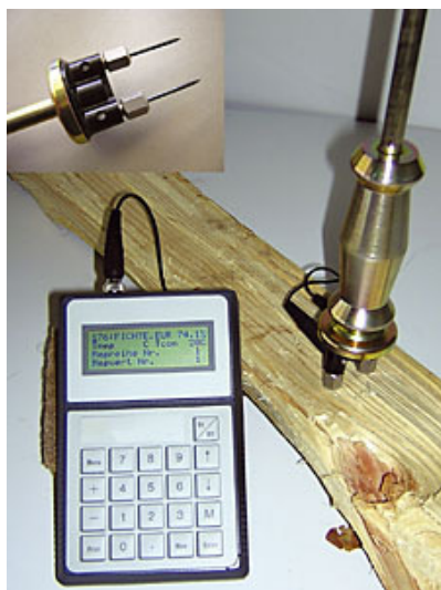
Figure 2.8: Wood moisture meter with electrodes
