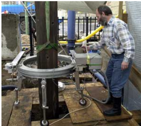
Figure 2.13: Mobile computer tomography on wooden foundation piles
