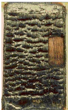
Figure 1.71: Heat-insulating foam layer of chemical fire protection cladding
