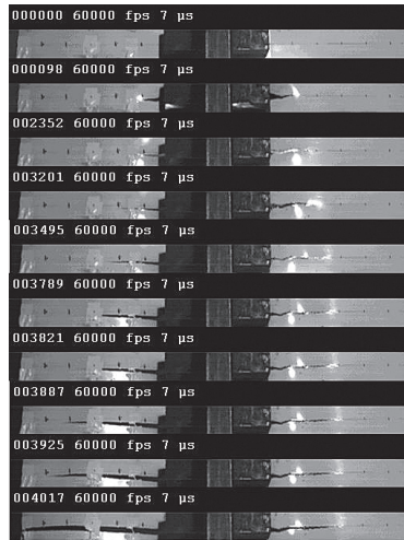
Figure 5: Crack propagation snapshots.
