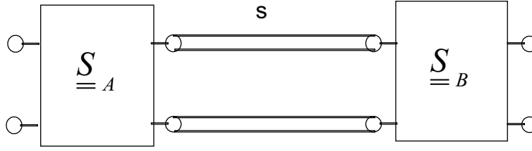
Figure 9.3: Fundamental mode equivalent circuit of the stub
